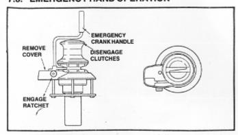
In the event of a power or control failure, engage the spring ratchet. Disengage the clutch and remove the chain pipe cover. Fit the emergency hand wind crank into its hole until fully home. Wind handle anticlockwise to recover chain and anchor. The ratchet will prevent the gipsy from running back out.
