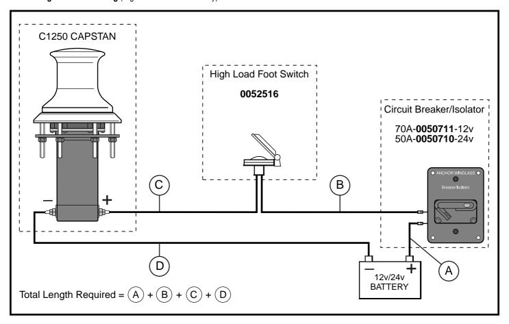
Note: Reversing polarity will result in permanent damage to the capstan (see 5.2.1). ALL installations must be carried out in accordance with USCG, ABYC and NMMA requirements. If you have any questions regarding this installation contact nearest Simpson-Lawrence Agent.
