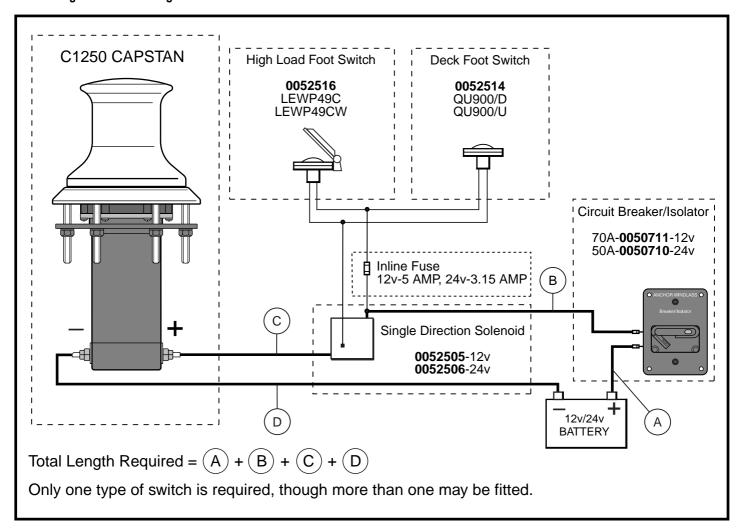
**Note**: Reversing polarity will result in permanent damage to the capstan (see **5.2.1**). ALL installations must be carried out in accordance with USCG, ABYC and NMMA requirements. If you have any questions regarding this installation contact nearest Simpson-Lawrence Agent.
