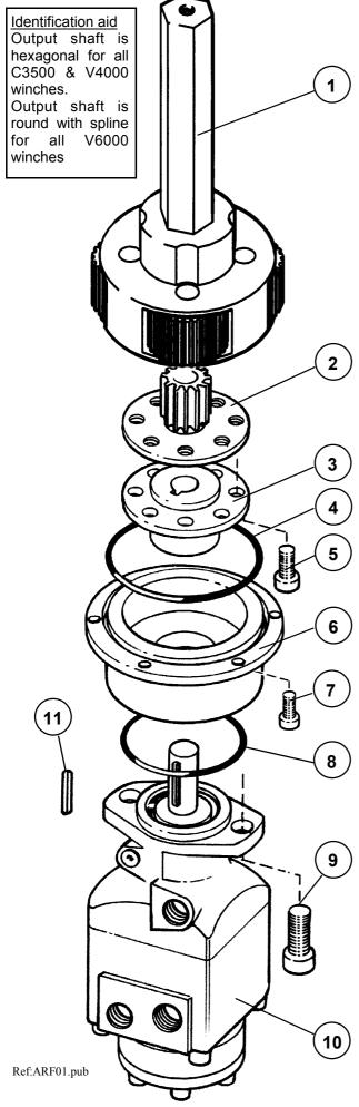
Transmission Parts List C3500ARF Capstan V4000GARF, V4000GDARF Windlass V6000GARF, V6000GDARF Windlass
