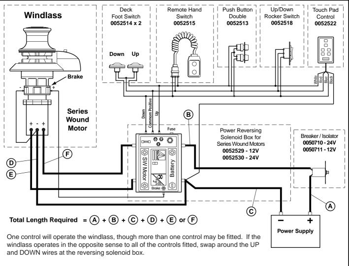
**NOTE:** Electric brake **must** be wired, otherwise windlass will be damaged (see **5.2**.3). ALL installations must be carried out in accordance with USCG, ABYC and NMMA requirements. If you have any questions regarding this installation contact nearest Simpson-Lawrence Agent.
