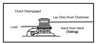
If the gipsy is in use it should be locked by its ratchet. Slacken the clutch nut to enable the drum to rotate independently of the gipsy. Wrap at least three coils of rope, loosely, around the drum clockwise to avoid it slipping. Apply a light hand pressure on the *tail* of the warp and apply power. While the windlass rotates under power, *tail* the warp hand over hand until the task is complete. Secure the warp after use.
